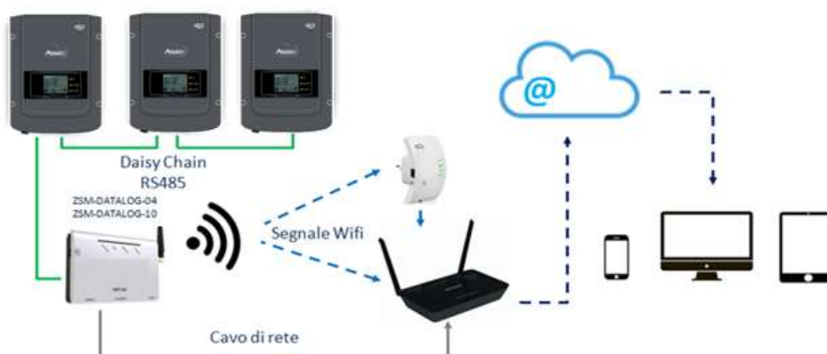
Figure 77 – Diagram for connecting the ZSM-DATALOG-04 / ZSM-DATALOG-10 datalogger
