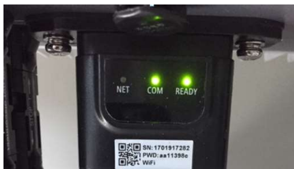
Figure 73 - Initial status of LEDs
