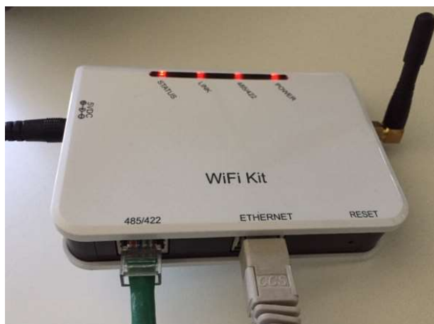
Figure 85 – Ethernet cable connected to the datalogger
