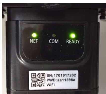
Figure 75 - Irregular communication status between inverter and adapter
