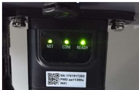
Figure 74 - Final status of LEDs
